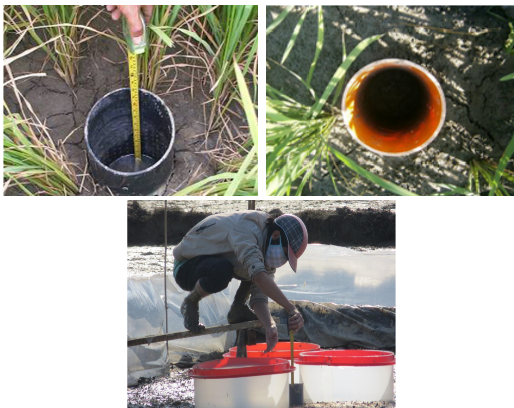
Figure 7.1. PVC pipes with multiple holes on the sidewall that installed in a paddy soil to monitor the surface water depth.
