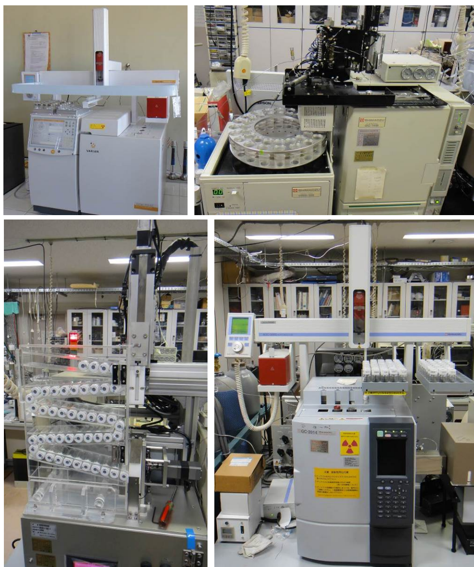
Figure 5.5. Examples of automated gas injection systems for glass vials.
