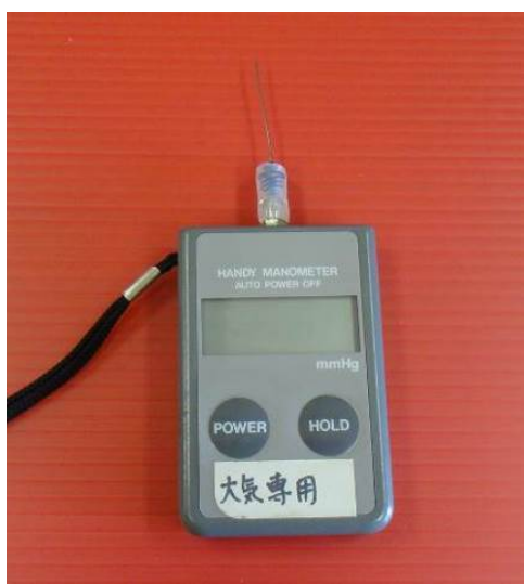
Figure 4.8. A portable manometer. The needle is inserted into an evacuated vial through a rubber stopper to check the degree of vacuum.
