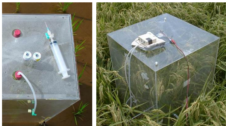
Figure 4.5. A plastic syringe (left) and a battery-operated pump (right) for gas collection.
