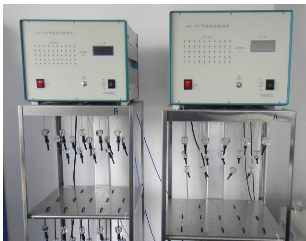
Figure 5.6. An example of automated gas injection system for plastic bags.
