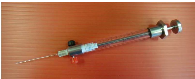
Figure 5.3. A gas-tight glass syringe with an open-shut valve.
