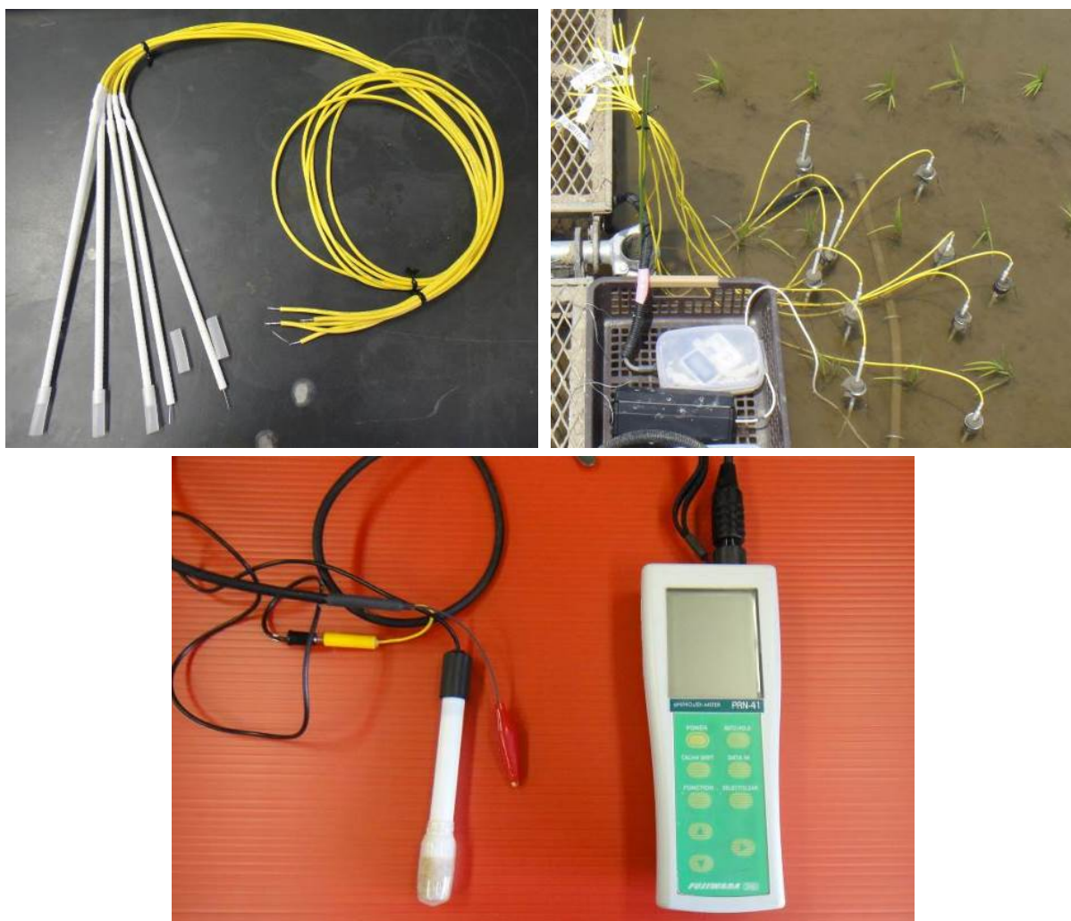
Figure 7.3. Platinum-tipped electrodes (left), electrodes installed in a flooded paddy soil (right), and a portable redox potential meter (bottom).
