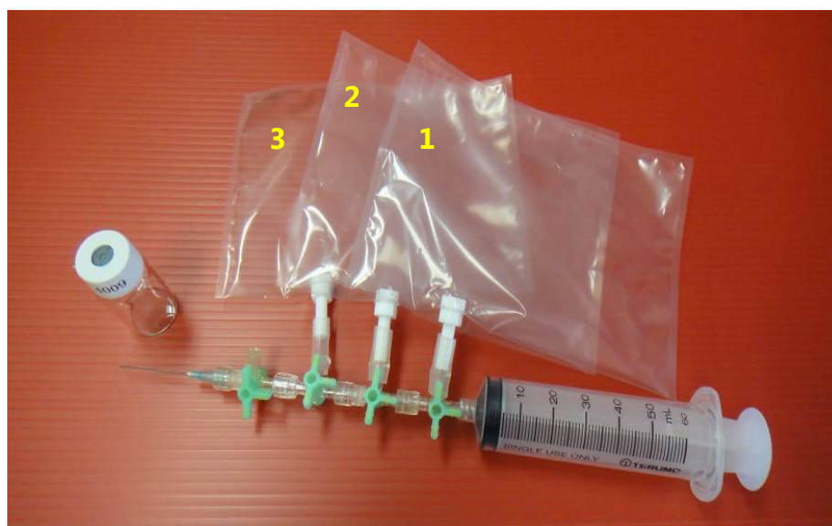
Figure 5.7. A gas dilution tool consisting of a plastic syringe and three plastic bags. Bag 1 contains an inert gas; bag 2 contains a high-concentration standard gas; and bag 3 receives the diluted gas (low-concentration standard gas).
