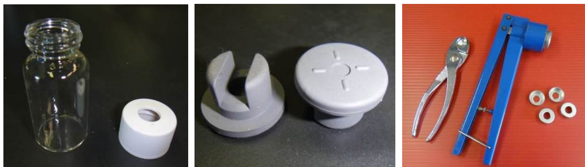
Figure 4.7. A glass vial and plastic screw cap (left); butyl rubber stoppers (middle); and aluminum caps, crimper, and decapper (right).
