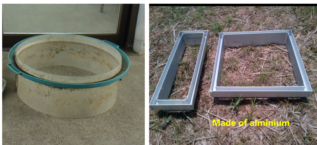
Figure 3.4. Examples of bases for chambers with round and rectangular footprints.
