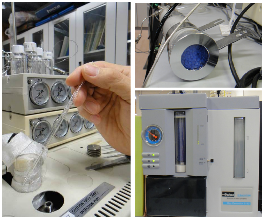
Figure 5.2. Examples of GC maintenance. Left, glass tube cleaning; top right, replacement of silica gel; bottom right, checking the water level in the hydrogen generator.
