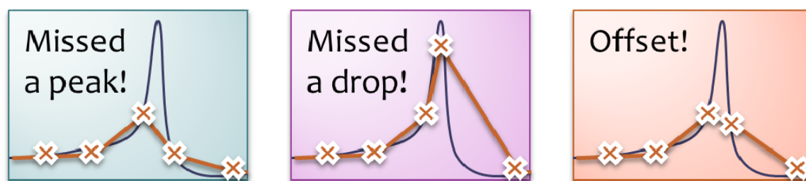
Figure 6.5. Examples of the consequences of inadequate gas sampling before and during agricultural management events.
